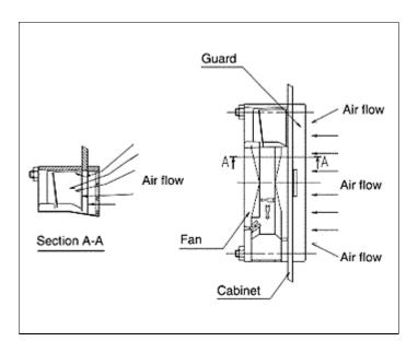
fig. 9 Air Flow in a traditional product on the market, as equipped with a resign Finger guard
