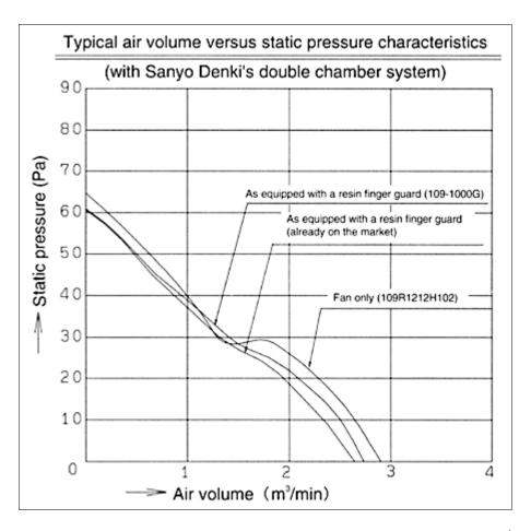
fig. 10 Air volume versus static pressure characteristics as equipped with a resin Finger guard (119mm sq.) as compared to one already on the market
