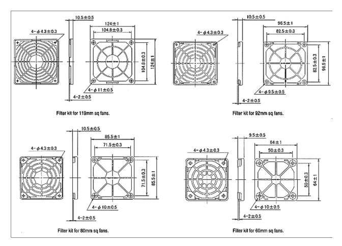
fig. 5 Outside dimensions of Filter kits
