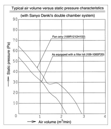
fig. 6 Typical air volume versus static pressure characteristics as equipped with a Filter kit (119mm sq.)
