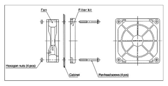
fig. 4 How to install the new product
