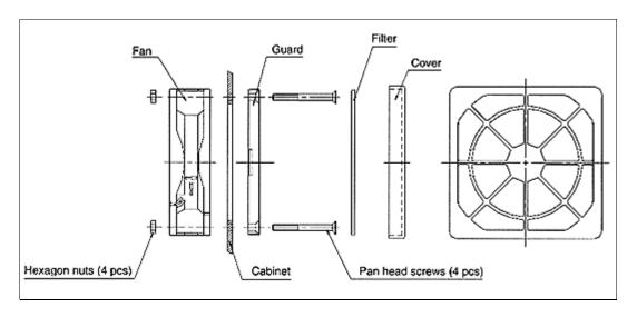
fig. 3 How to install traditional models
