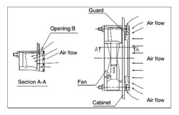
fig. 8 Air flow in the new product as equipped with a resign Finger guard
